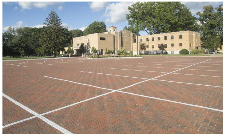
Description: Clay brick paver with chamfered edges and spacer lugs, 4"x8"x2-3/4", Red blend City Line Series Pavers by Belden Brick Company, [www.beldenbrick.com](http://www.beldenbrick.com)
