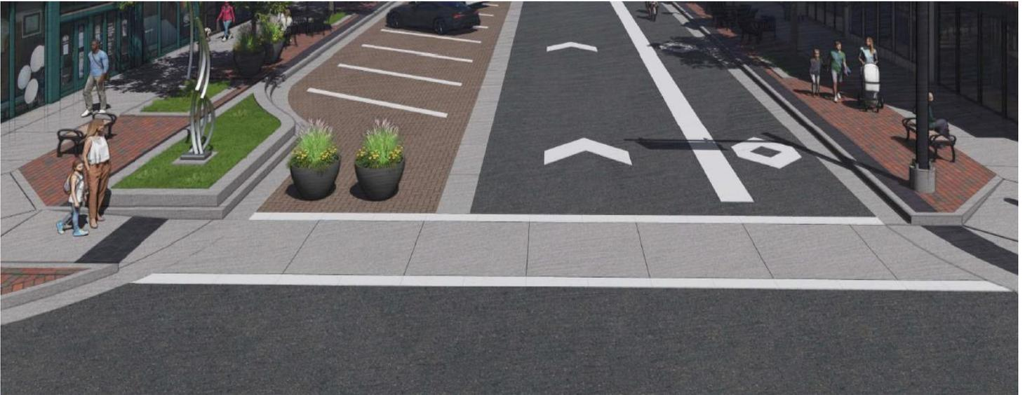
Concrete crosswalk pavement (8' wide) with painted white stripes (12" wide) on each side of the concrete surface to delineate the crosswalk and meet safety standards
